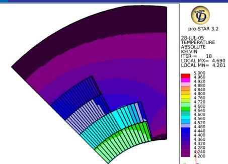
Uniform Volumetric heat source ----- 0.1WAmbient temperature 4.2 K Constant material properties for T = 5K
