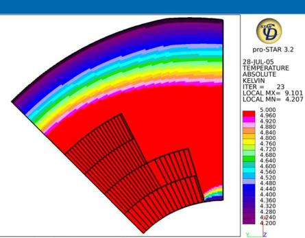
Uniform Volumetric heat source ----- 1WAmbient temperature 4.2 K Constant material properties for T = 5K
